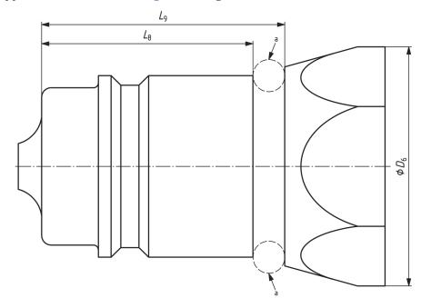
Shape of neck between  $L_8$  and  $L_9$  is optional but shall be circular to accommodate dust sealing.
